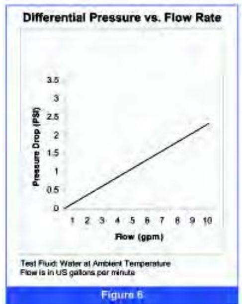
sus flow rate all compare very favorably with standard string wound cartridges. The test cartridge is of 10 inch nominal length and 2½ inch diameter.
