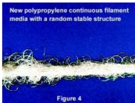
Each of the polypropylene filaments in the new media continues, without a break, throughout the length of the yarn, making the cartridge free from any media migration problems. There are no short fibers. The continuous filaments are melt-spun (extruded) by a newly developed method in which no spin-fish chemi-
